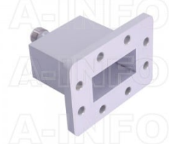
187WECAN Endlaunch Rectangular Waveguide to Coaxial Adapter 3.95-5.85GHz WR187 to N Type Female
